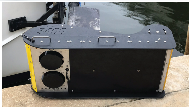
4. Large Multi-Channel Hydrophone can be Configured in "Pipe Line Finder Mode"
